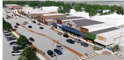
two lanes of traffic each way, center turn lanes, medians, and sidewalks, with the design centered on safety, function, and Sioux Center's character. See concepts at [www.siouxcenter.org/highway75](http://www.siouxcenter.org/highway75)
